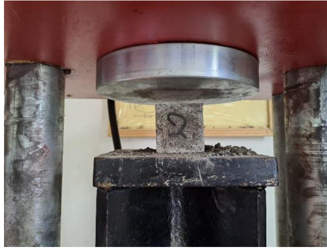
Fig. 3. Compressive strength testing [34,46,47]
