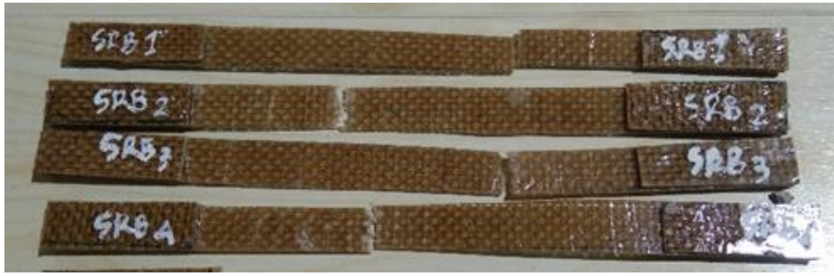
Fig. 6. Failure modes of RFRP under tensile test
