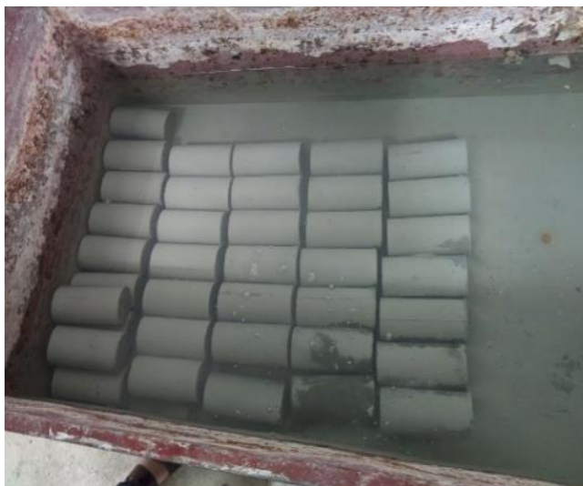
Fig. 11. Curing of some concrete cylinder specimens
