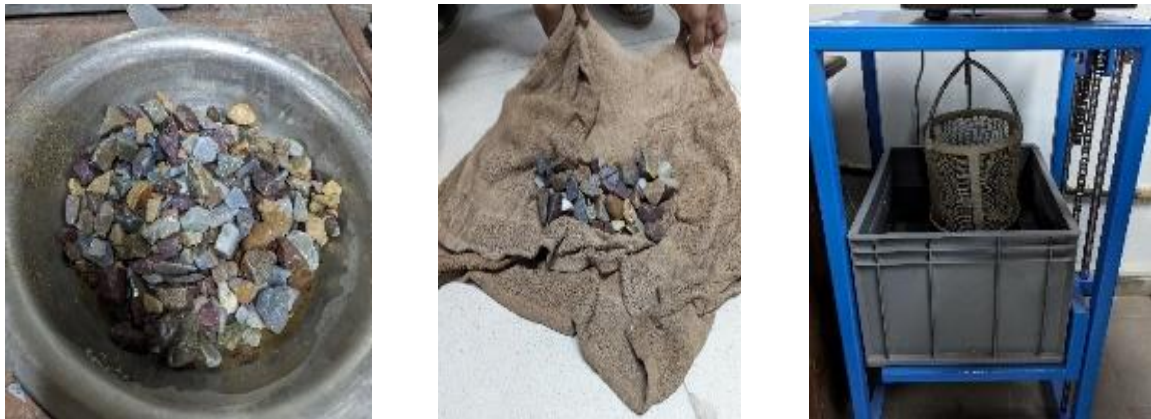
Fig. 5. Specific gravity and absorption capacity of coarse aggregate
