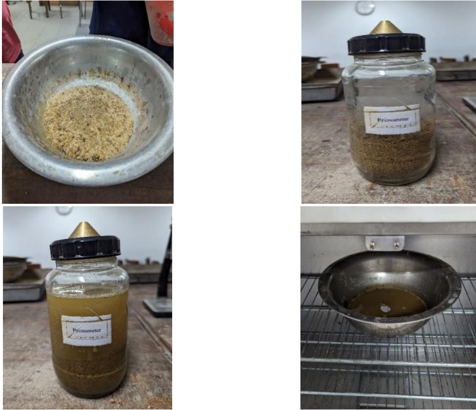
Fig. 6. Specific gravity and absorption capacity of sand
