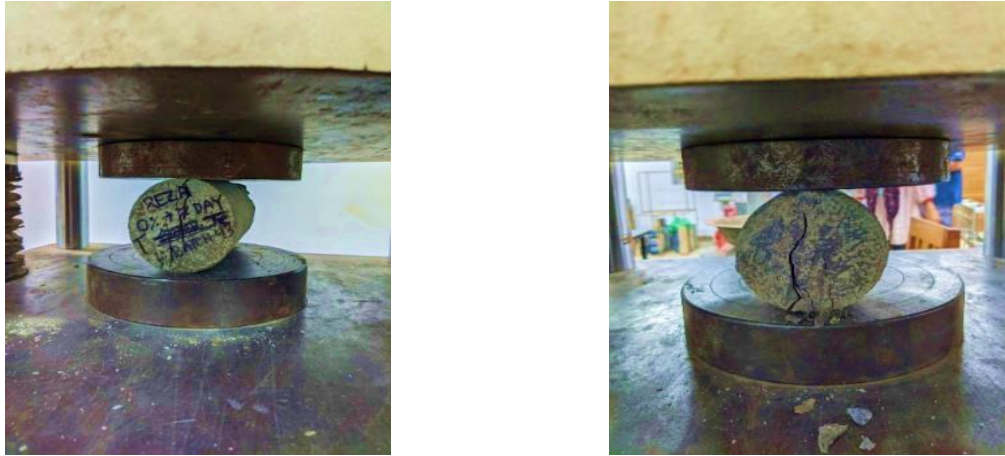
Figure 14. Split tensile strength test
