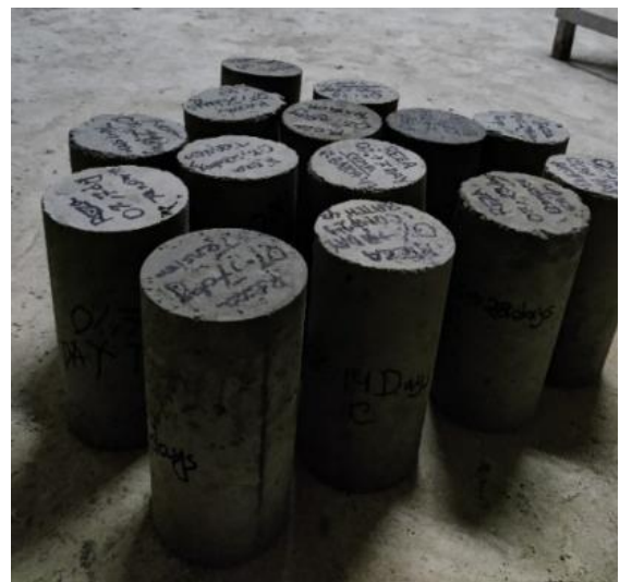
Fig. 12. Concrete cylinder specimen after 28 days of curing
