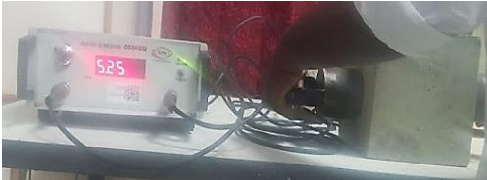
Fig. 9. UPV test set-up
