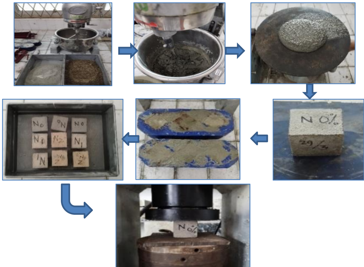
Fig. 2. Test specimen manufacturing procedure
