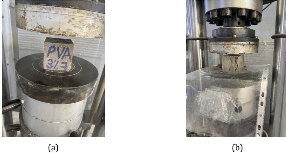
Fig. 4. (a) Compression cubic before failure and (b) The cubic After failure
