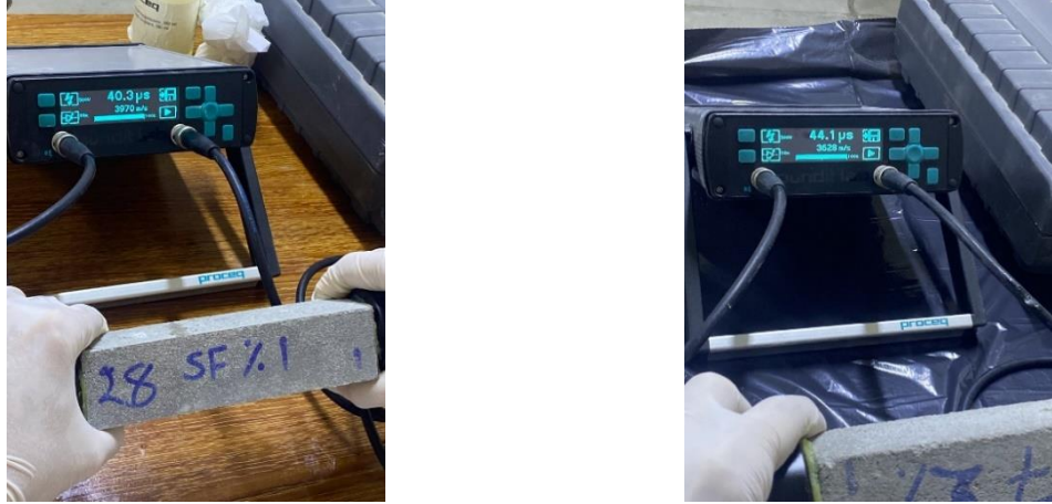
Fig. 11. The sample during test in UPV devise
