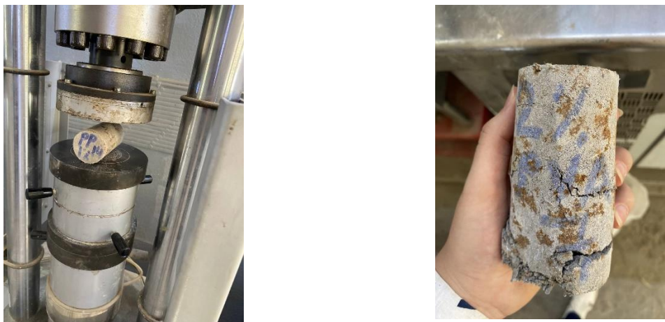
Fig. 14. The cylinder before and after failure
