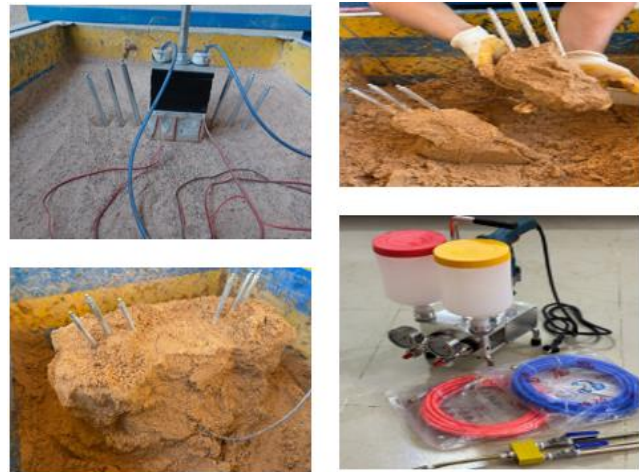
Fig. 7. The pipes injection and the PU machine.
