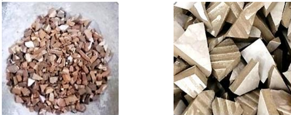
Fig. 2. Porcelain applied in concrete mixture
