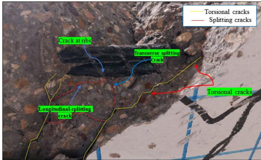
Fig. 13. Cracks types within splice region(G-Lap300)
