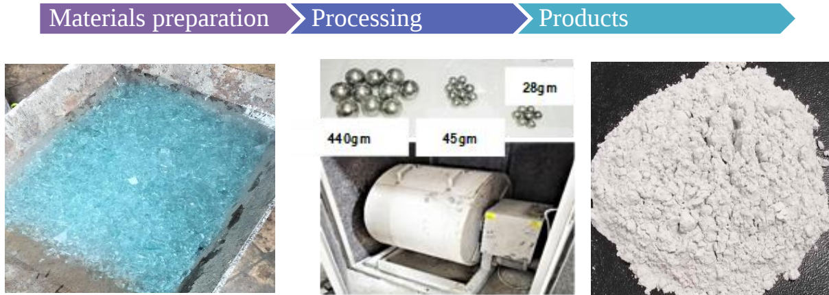
Fig. 2. Preparation of cementitious powder from WG
