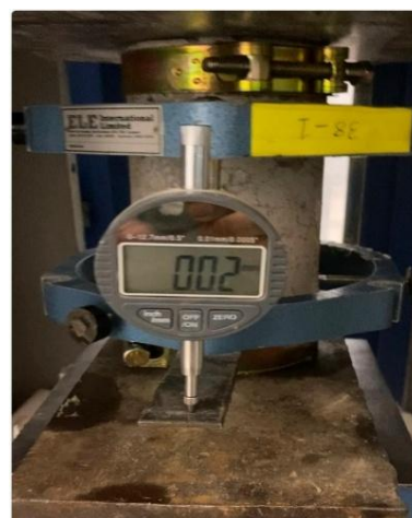
Fig. 3. Testing setup for the uniaxial compressive strength test
