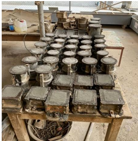
Fig. 1. Concrete specimens' preparation
