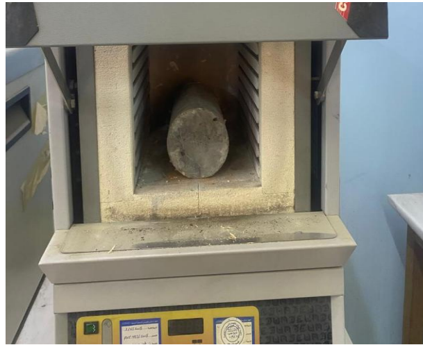
Fig. 2. Electric furnace used to expose the specimens to elevated temperature
