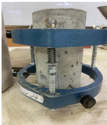
Fig. 3. Testing setup for the uniaxial compressive strength test
