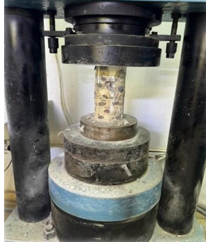
Fig. 11. Cores are being tested
