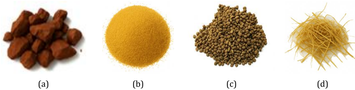
Fig. 3. Raw materials for manufacturing raw clay bricks (a) Clay (<0,075mm), (b) Dune sand (0-2mm), (c) Coarse sand (2-2.5 mm), and (d) Straw fiber (25-30 mm)
