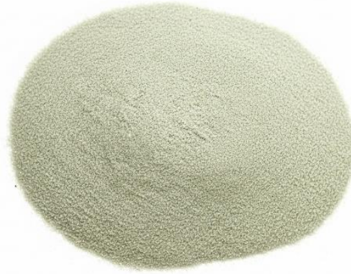
Fig. 1. Waste glass powder used in HVFA concrete mixture
