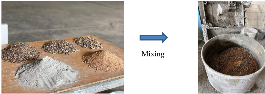
Fig. 5. Dry material (fly ash and aggregate) before and after mixing
