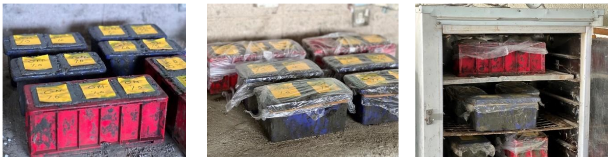
Fig. 7. The steps of curing geopolymer concrete mixes
