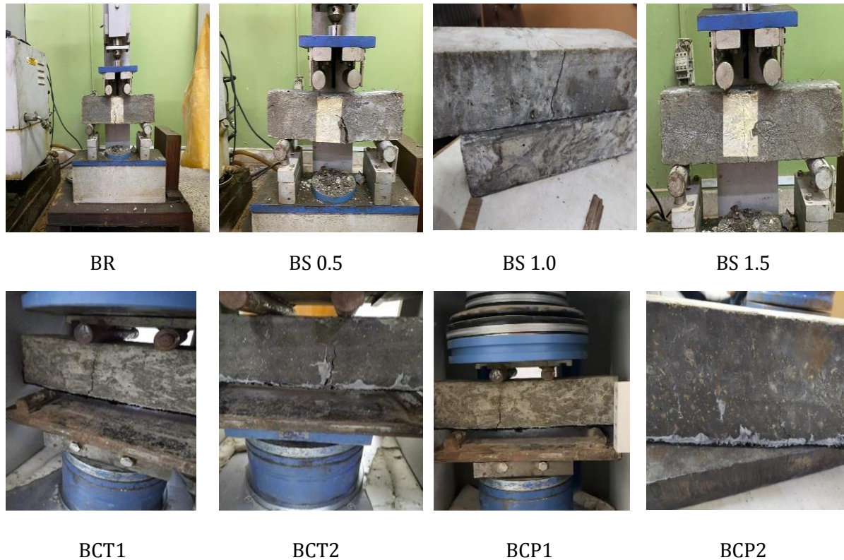
Fig. 7. Failure mode of tested specimens
