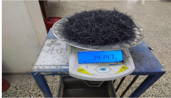
Fig. 1. Steel fiber used in specimens
