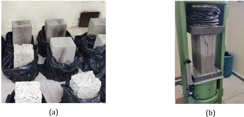
Fig. 13. Compressive Strength Test of Low Walls (a) Low walls and (b) Compression test of low walls
