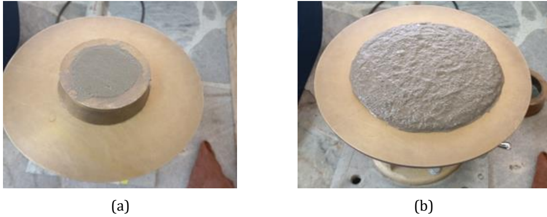
Fig. 7. Mortar flow test (a), Mortar in mold (b) Mortar on fluidity table
