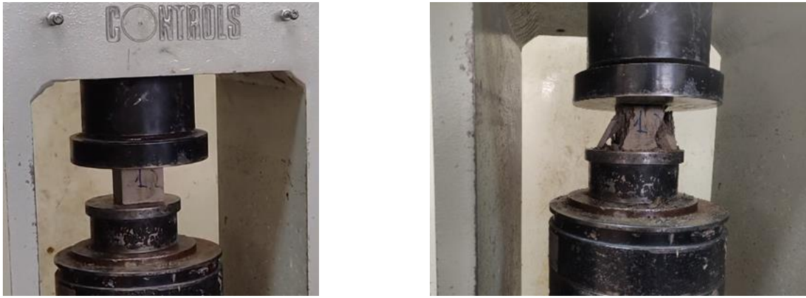
Fig 16. Compressive strength test of mortar cubes
