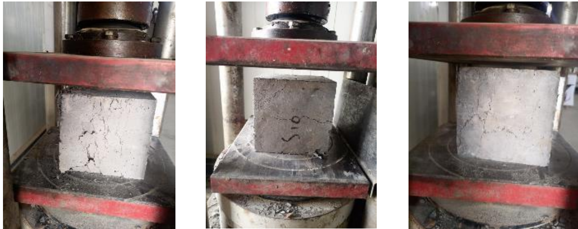
Fig. 13. Compressive strength failure for some specimens
