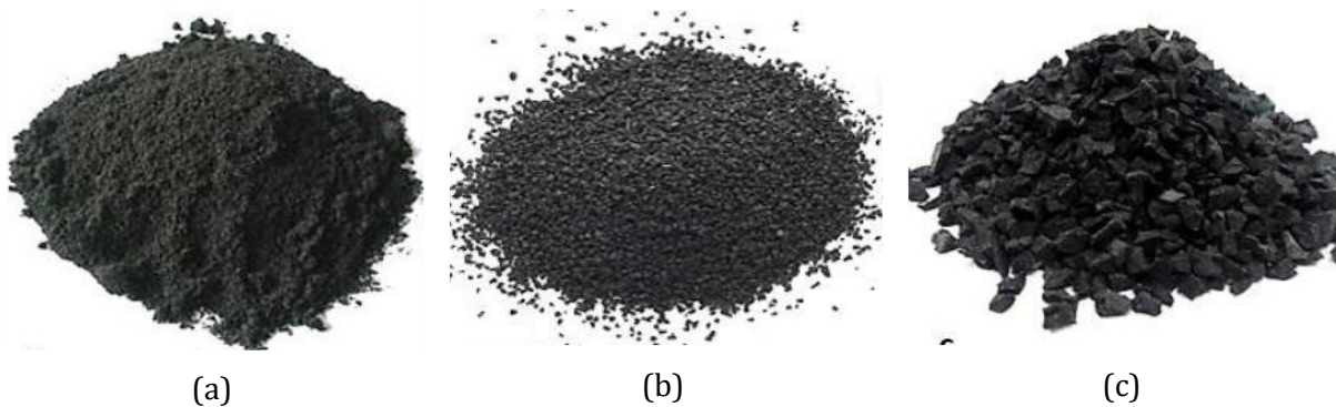
Fig. 2. Recycled scraped tyre rubber, which products from recycling factories (a) ground rubber, (b) crumb rubber and (c) chip rubber [9]
