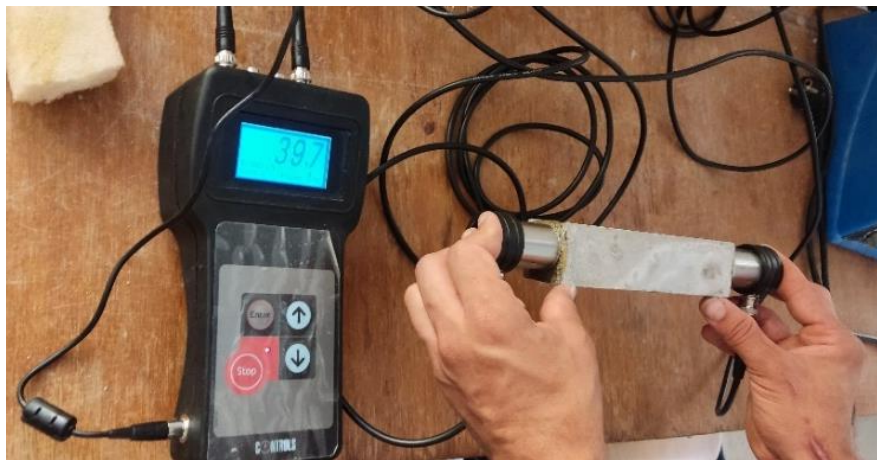
Fig. 16. Ultrasonic pulse velocity measurement in mortar specime
