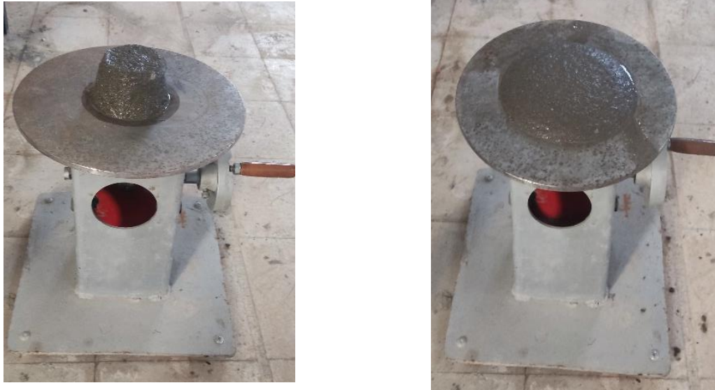
Fig. 11. Flow table apparatus and mortar spread
