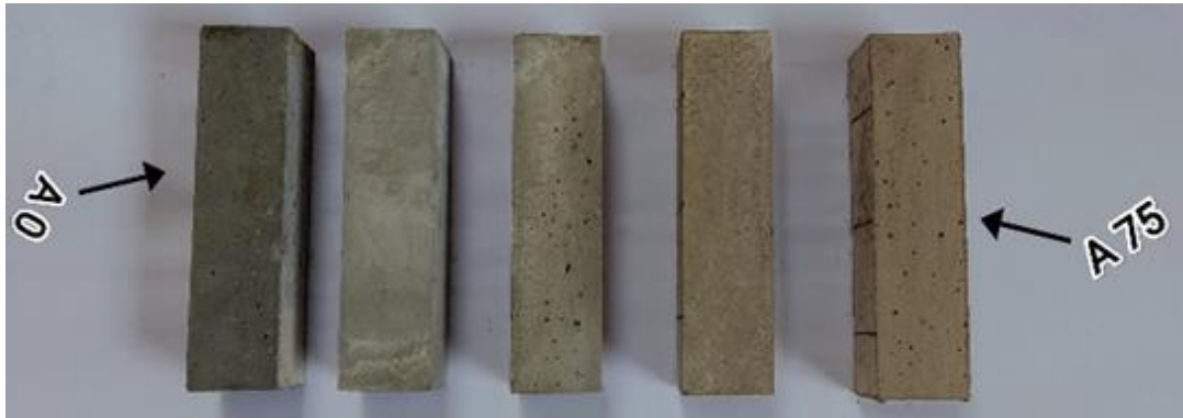
Fig. 12. Specimen appearance changes following SSA addition
