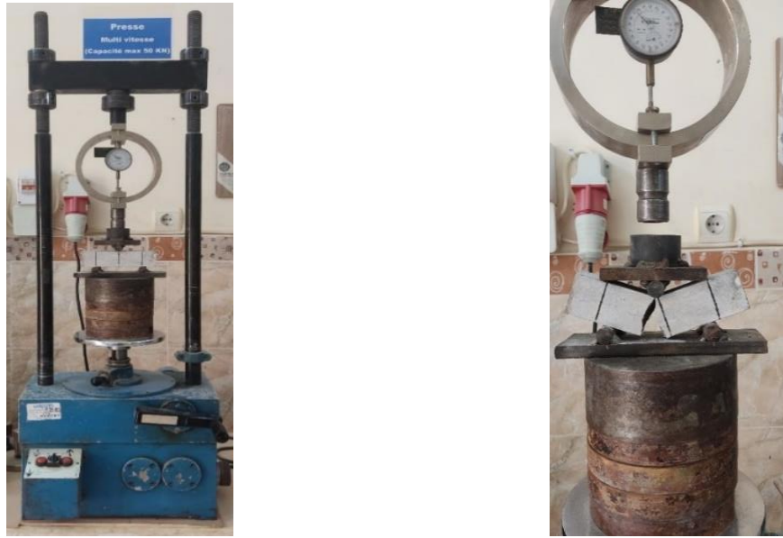
Fig. 6. Assessment of mechanical properties: a focus on flexural strength testing
