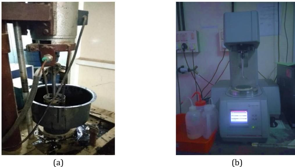
Fig. 1(a). Cowls' blade mechanical shaker and (b) Dynamic Shear Rheometer (DSR)
