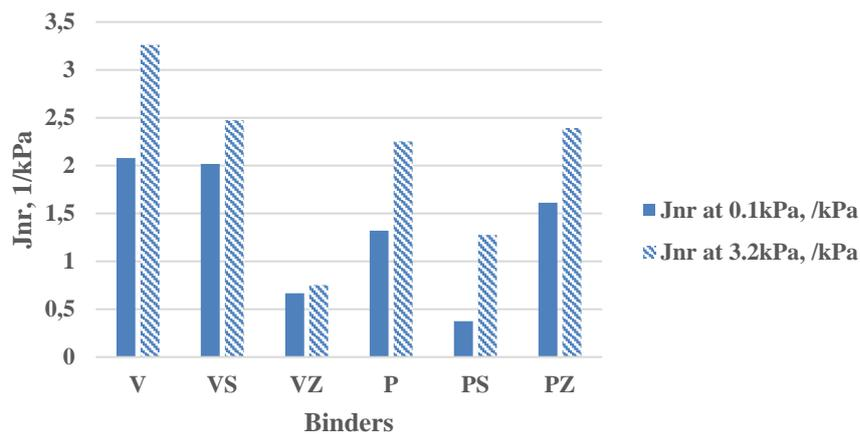
Fig. 7. Variation of Non recoverable creep compliance values (Jnr) for the binders
