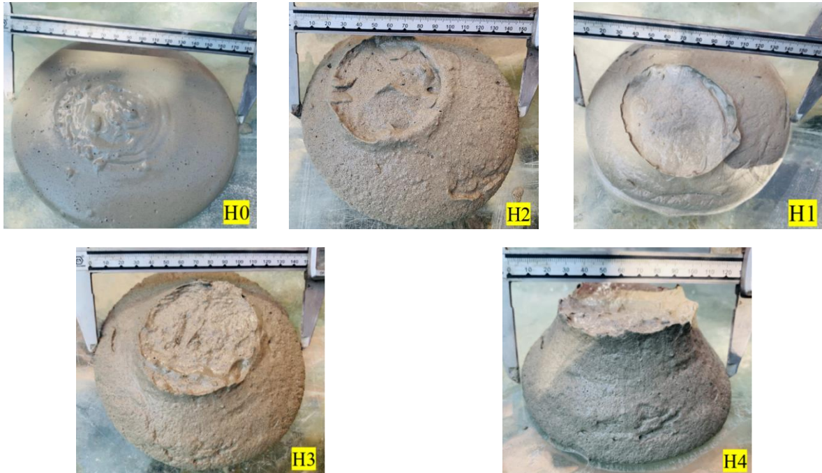
Fig. 4. Fresh foamed concrete slurry with different HEC content
