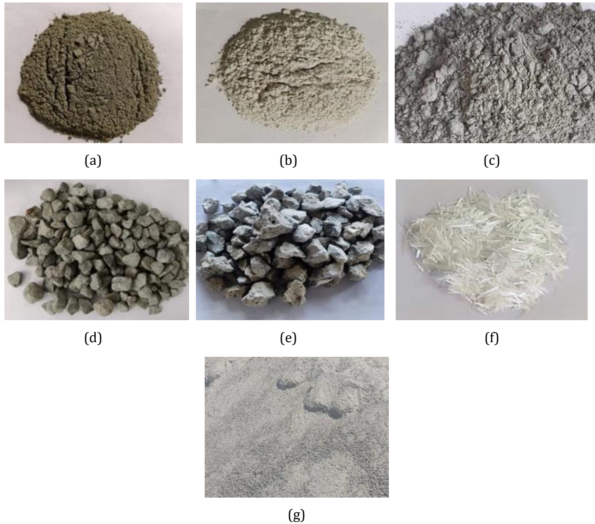
Fig. 3. Raw materials employed in the study: (a) OPC, (b) Alccofine, (c) PPC, (d) NCA, (e) RCA, (f) Glass fibers, (g) M-sand
