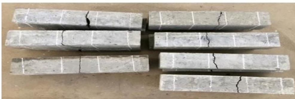
Fig. 9. Typical failures of prisms under flexure
