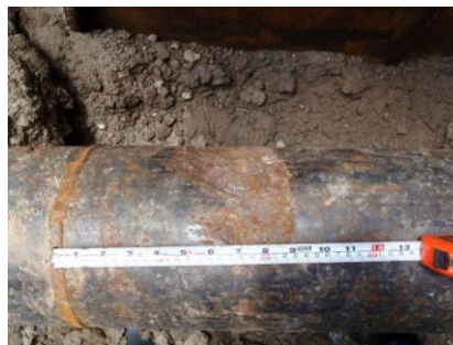
Fig. 2. An excavated gas pipeline subject to external corrosion [16]
