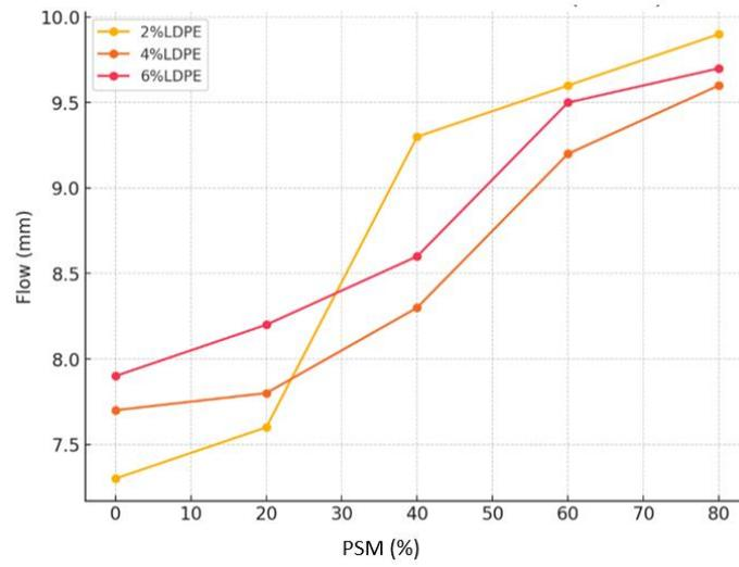
Fig. 5.: Flow versus percentage PSM
