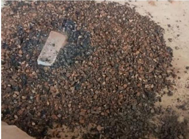
Fig. 1. Pulverized surface dressed pavement material
