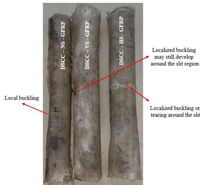
Fig. 8. Failure mode of the GFRP wrapped circular column with and without deficient
