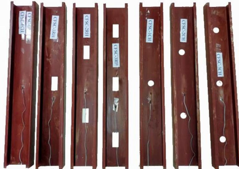
Fig. 4. CFS Column specimens before testing
