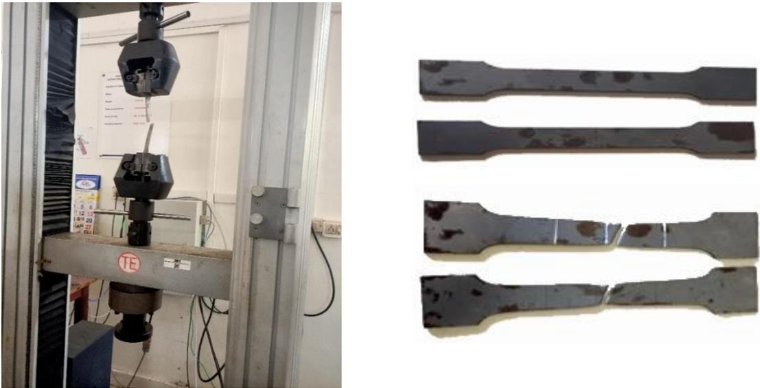
Fig. 2. Tensile test on CFS Coupon specimen
