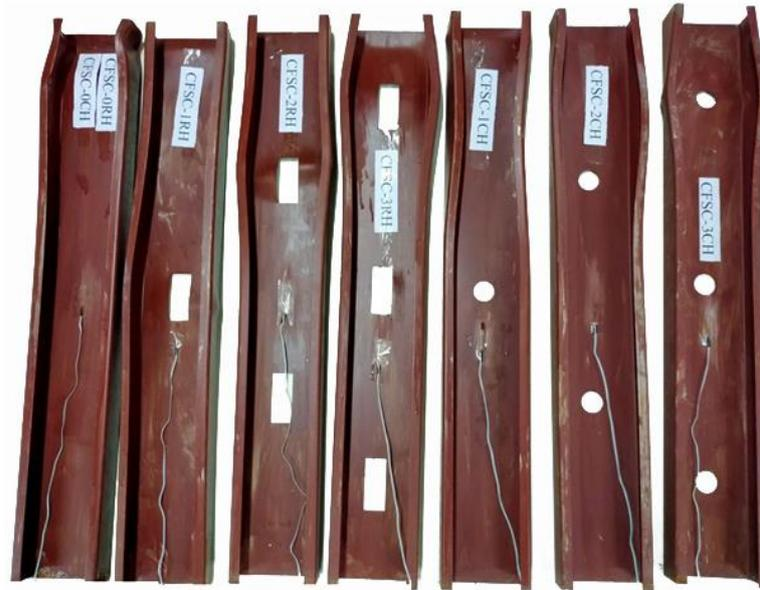
Fig. 10. Failure of the perforated CFS columns
