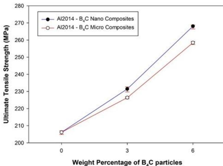
Fig. 8. Al2014 alloy ultimate strength vs nano and micro  $\text{B}_4\text{C}$  composites
