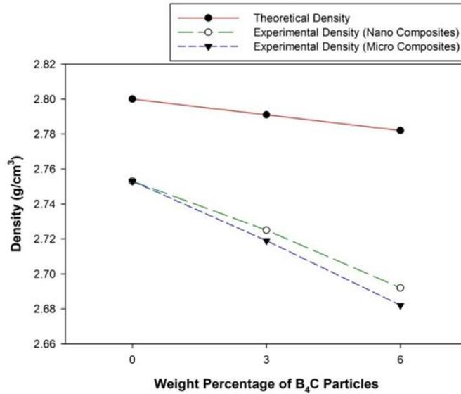
Fig. 6. Comparison of densities of Al2014 alloy with nano and micro B<sub>4</sub>C composites
