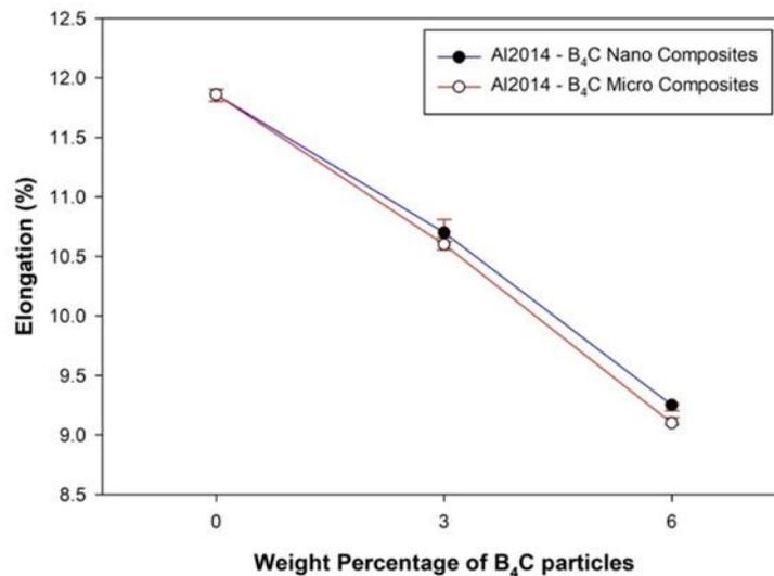
Fig. 10. Comparison of ductility of Al2014 with B<sub>4</sub>C composites
