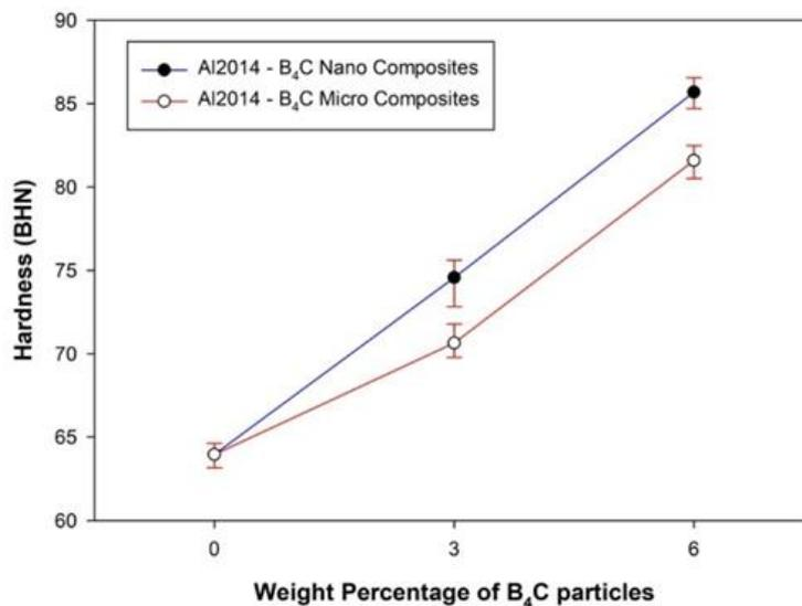
Fig. 7. Comparison of hardness of Al2014 alloy with nano and micro B<sub>4</sub>C composites
