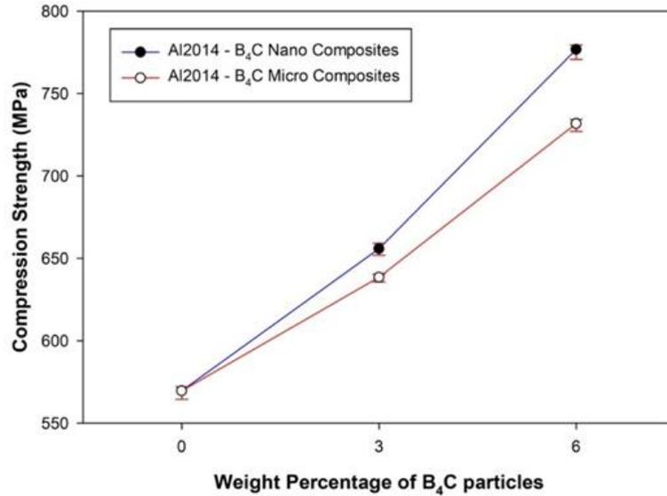
Fig.11. Al2014 alloy compressive strength vs. nano and micro B<sub>4</sub>C composites
