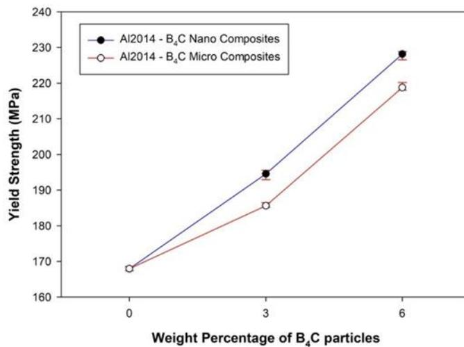
Fig.9. Al2014 alloy yield strength vs. nano and micro B<sub>4</sub>C composites
