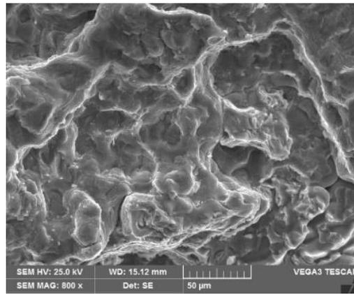
Fig. 12. Tensile fractured surfaces (a) Al2014 alloy (b) Al2014 – 6 wt. % of 200 nm B<sub>4</sub>C (c) Al2014 – 6 wt. % of 25 micron B<sub>4</sub>C composites
