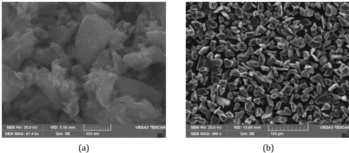
Fig. 1. SEM micro-photographs of (a) 200 nano-meter (b) 25-micron sized B<sub>4</sub>C particles
