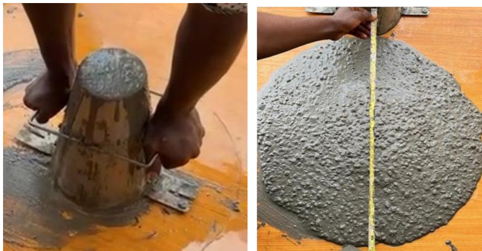
Fig. 1. Slump flow testing of the fresh concrete
