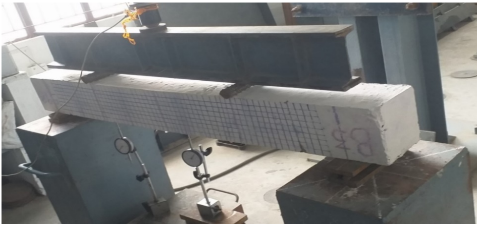
Fig. 9. Experimental setup of RC beam
