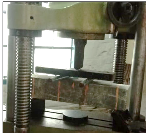
Fig. 6. Flexural strength test
