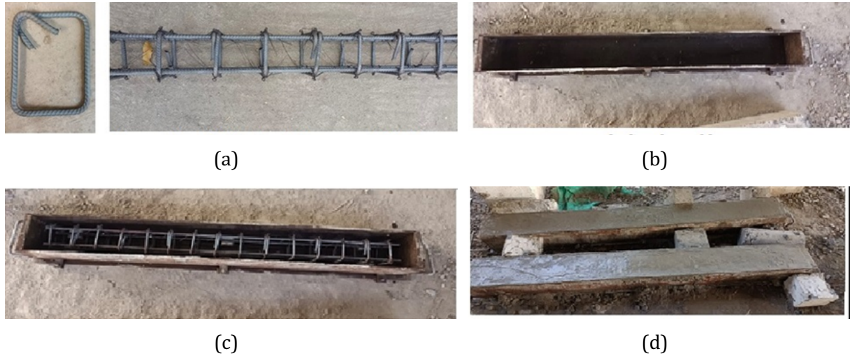
Fig. 7. Fabrication of the RC beams (a) Cross-section and longitudinal reinforcement details, (b) Steel mould, (c) Steel mould with reinforcement cage, and (d) Casting RC beams
