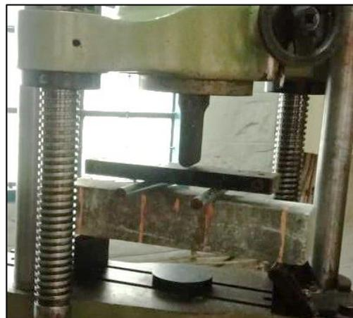
Fig. 6. Flexural strength test
