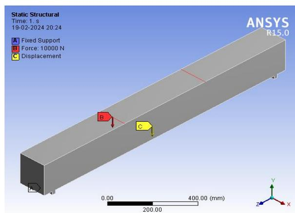
Fig. 12. Load and support arrangement of RC beam
