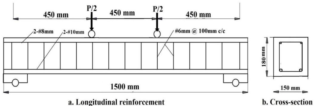
Fig. 8. Loading positions, cross-section and longitudinal reinforcement details of the RC beam
