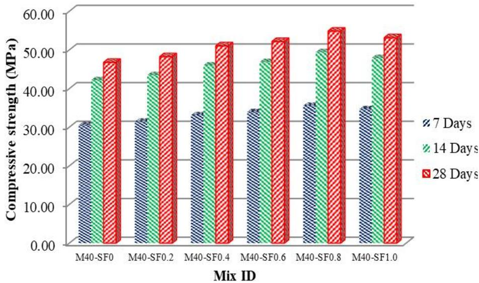
Fig. 13. Compressive strength of SFC at various ages
