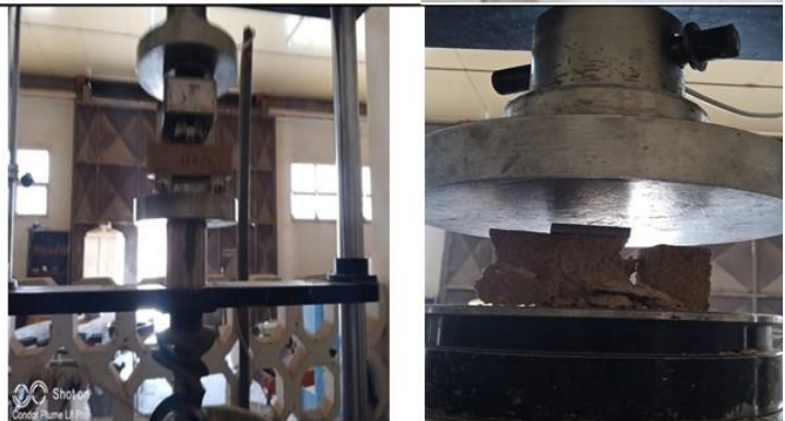
Fig. 2. Images illustrate the preparation and testing of geopolymer mortar (GPM)
