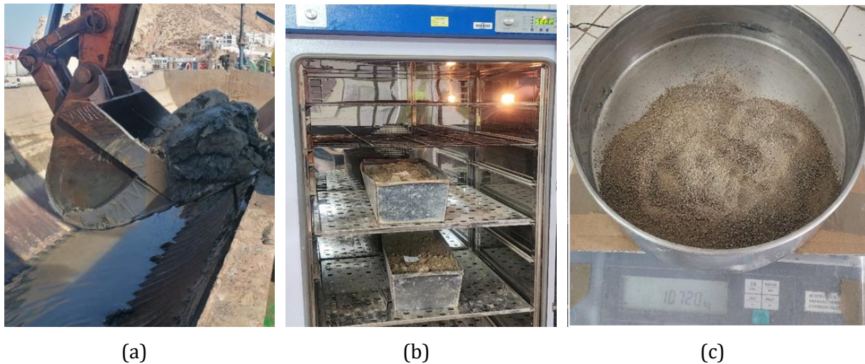
Fig. 3. Stages of Marine Dredged Sediment Collection and Processing: (a) Excavator scooping dredged sediment from the water at the port, (b) Sediment samples placed inside a drying oven for moisture removal, (c) Weighing the dried sediment using a balance scale.
