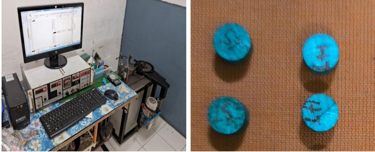
(a) (b) Fig. 4. (a) Pin on Disc wear testing machine (b) wear test sample
