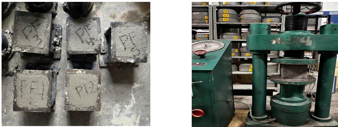
Fig. 3. Compressive strength test setup
