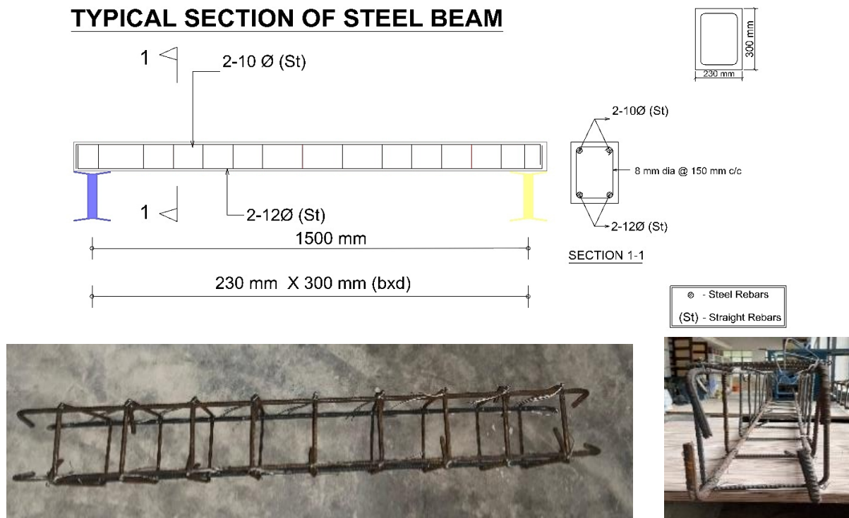
Fig. 4. Reinforcement detail of Steel beam
