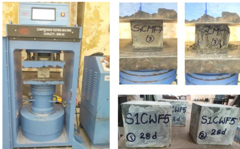
Fig. 7. Arrangement for compressive strength testing
