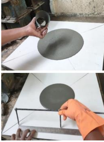
Fig. 4. Slump cone test
