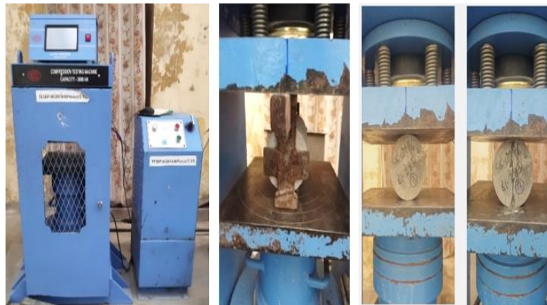
Fig. 8. Test setup of split tensile strength
