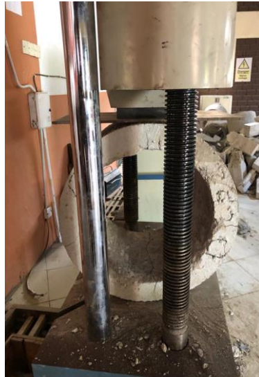
Fig. 5. Testing of concrete culvert
