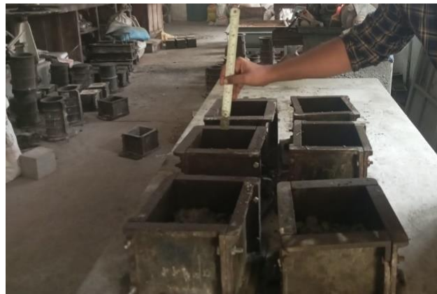
Fig. 4. Casting of layered cubes
