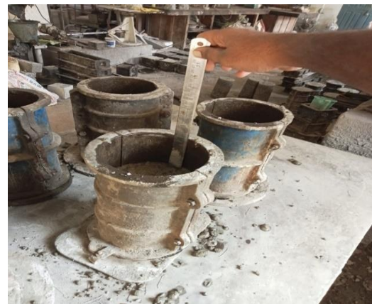
Fig. 8. Casting of layered cylinder
