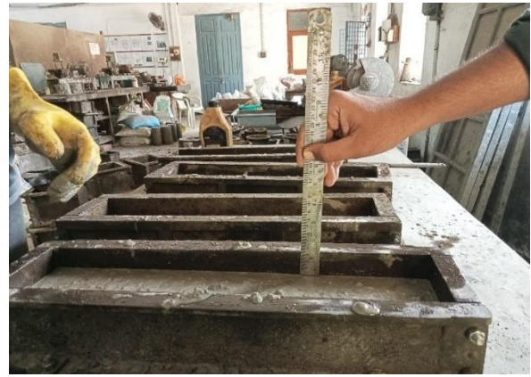
Fig. 12. Casting of layered Prism
