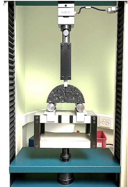
Fig. 30. Crack length recording under three-point bending test
