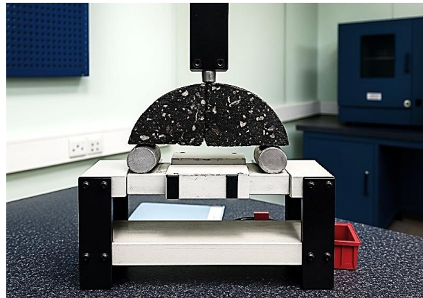
Fig. 7. The semi-circle specimens in laboratory
