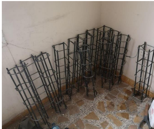
Fig. 4. Reinforcing steel cages of square and circular columns
