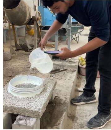
Fig. 5. Infiltration test of Pervious concrete slab
