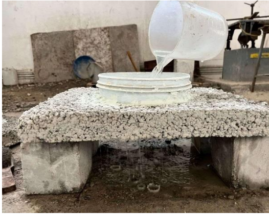
Fig. 5. Infiltration test of Pervious concrete slab
