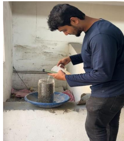
Fig. 7. Infiltration test of Pervious concrete cylinder
