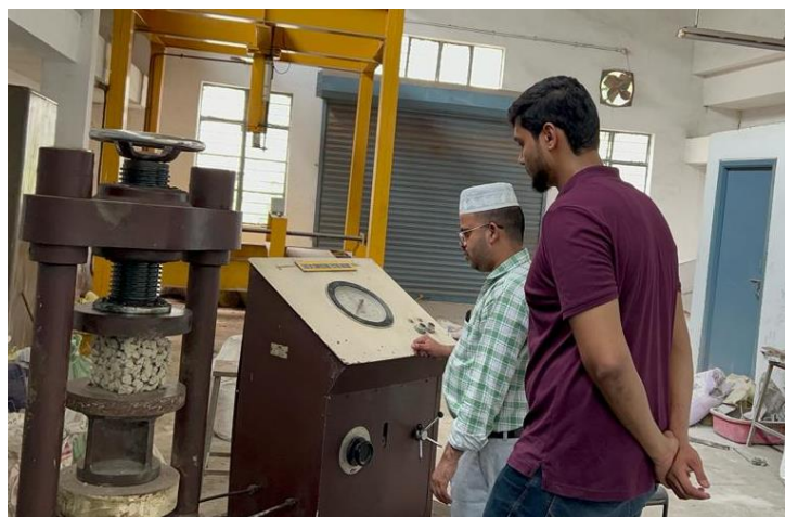
Fig. 4. Compressive test on Cube Specimens
