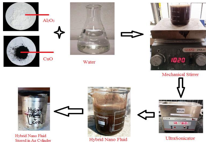
Fig. 4. \text{Al}_2\text{O}_3 – \text{CuO} based (at 50:50 ratio) hybrid nano fluid formation by two step method
