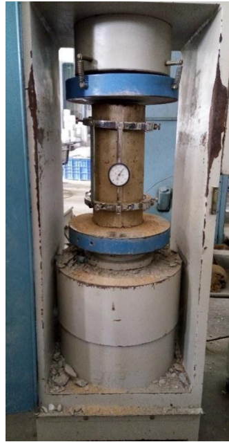
Fig. 4. Extensometer setup with compressive testing machine
