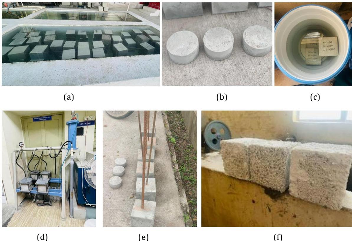
Fig. 5. (a) Curing of specimen (b) specimen for RCPT (c) specimen immersed in magnesium sulphate solution (d) specimen subjected to water permeability test (e) bond strength specimen (f) specimen after exposure to acid attack
