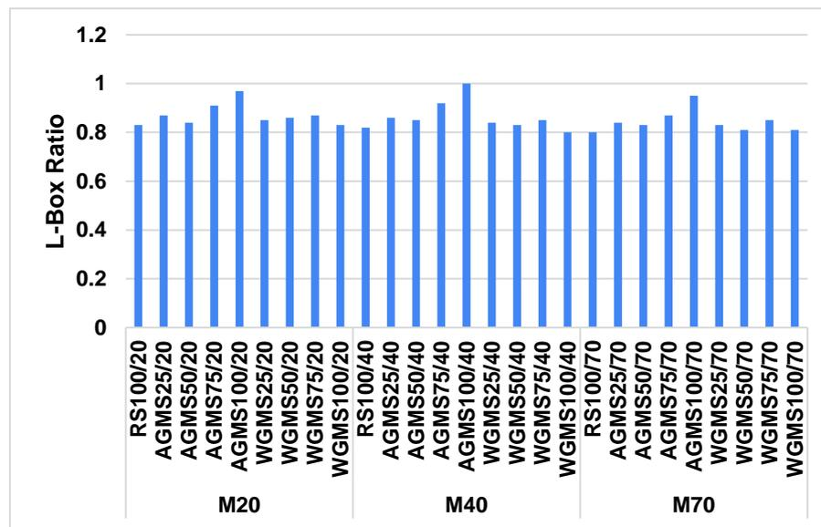
Fig. 9. L-Box Ratio for M20, M40 and M70 grade SCC using RS, AGMS ad WGMS
