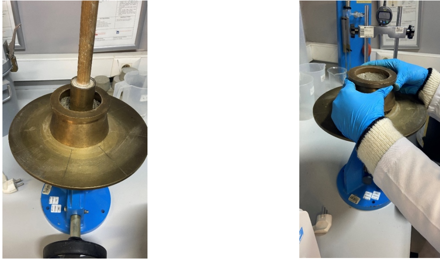
Fig. 1. Slump flow experiment conducted on fresh geopolymer mixtures
