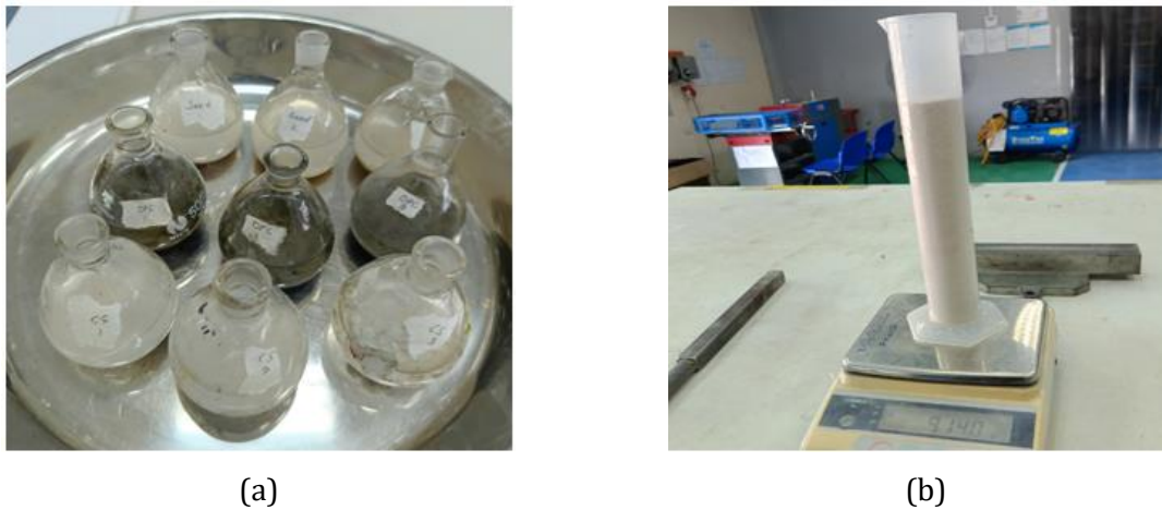
Fig. 2. (a) Specific gravity test (b) density test
