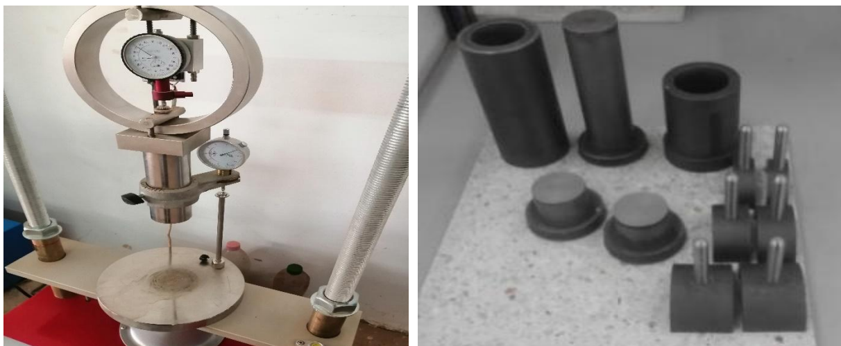
Fig. 9. unconfined compressive strength (UCS) testing apparatus: load frame and split molds
