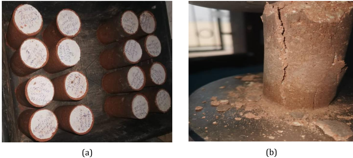
Fig. 10. (a) Samples for different durations: 3, 7, 14, and 28 days and (b) The crushing of the test pieces
