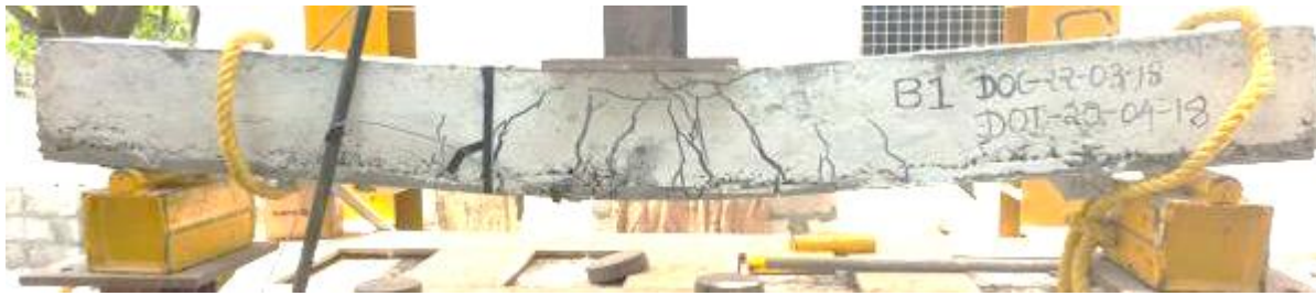
Fig. 13. Crack patterns and deflected shape [12]
