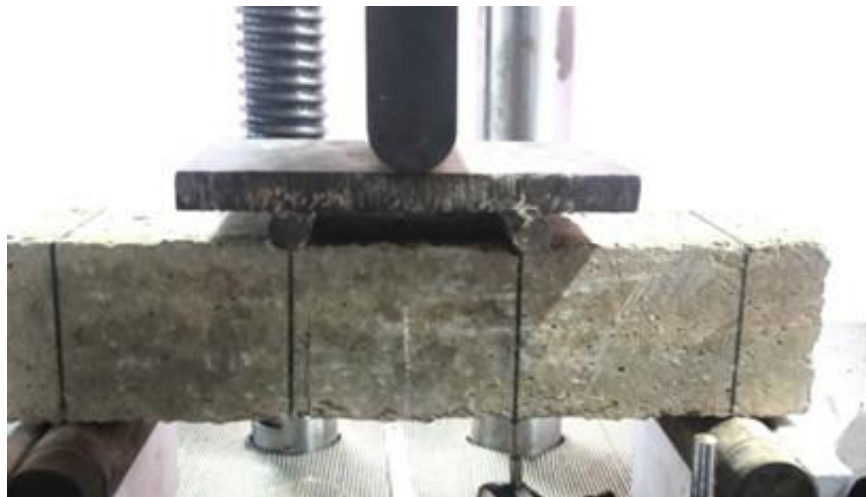
Fig.13. Crack pattern observed in prism made with colloidal silica from experimental investigation
