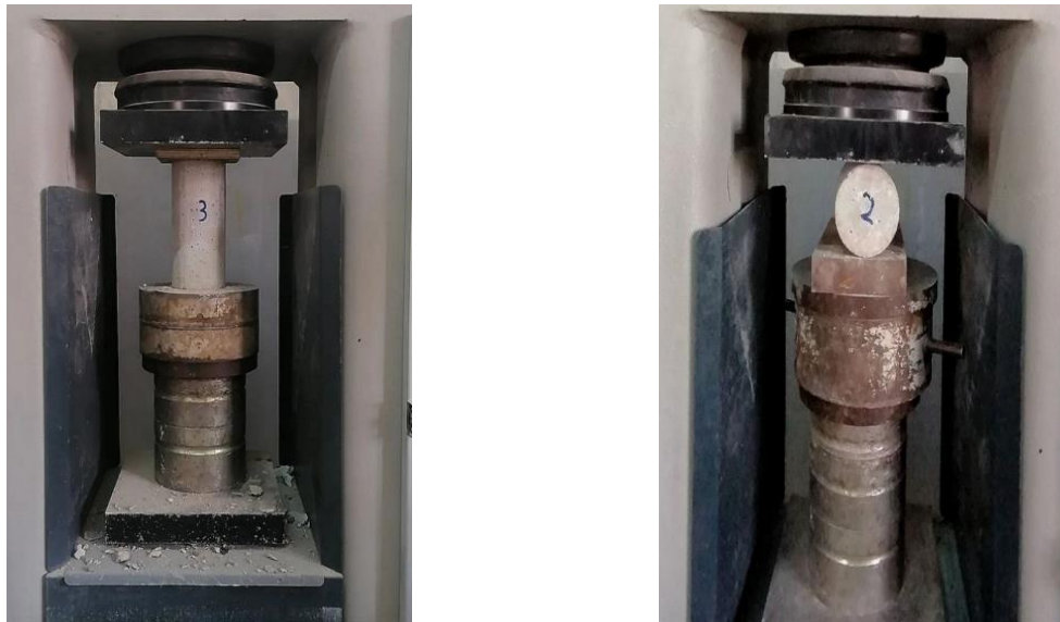
Fig. 2. Compressive and tensile test configurations
