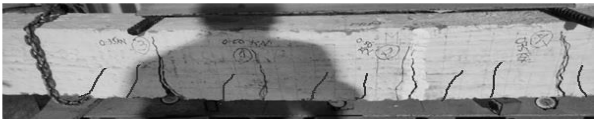
Fig. 7. Failure pattern of the reference beam
