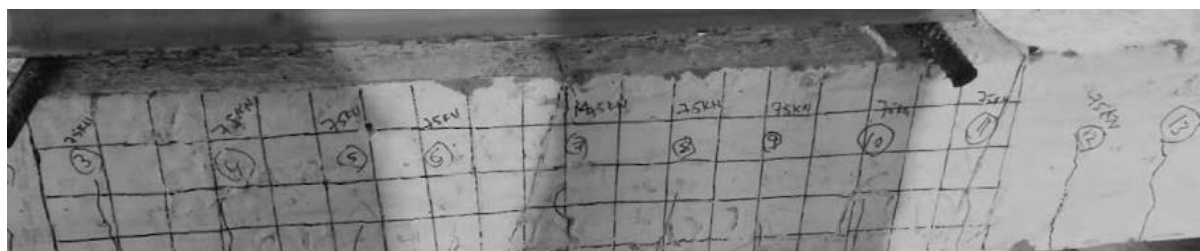
Fig. 8. Failure pattern of the CAZ beam
